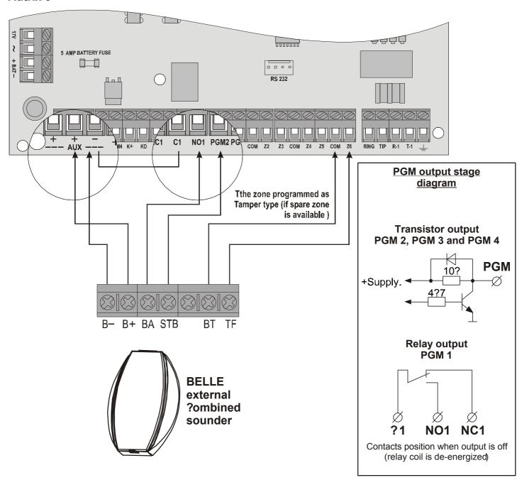
NOTE: PGM1 must be programmed as "External Bell". PGM 2 (in this example) must be programmed as "Follow Strobe".
