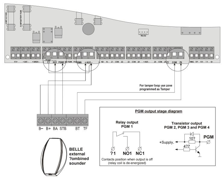
NOTE: PGM1 must be programmed as "External Bell". PGM 2 (in this example) must be programmed as "Follow Strobe".
