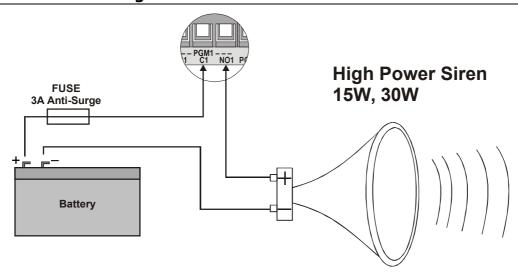
NOTE: When a high power siren is to be connected to the Matrix, the PGM1 (C1, NO1) output should be used. This output uses a relay to switch up to a maximum 3A dc current capacity, allowing the use of an additional battery to power the siren as shown in the diagram above.
