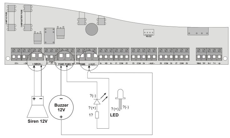
NOTE: If a monitored siren is not to be used, either programme PGM 7 as Not Used, or link out the + SIREN – terminals with a 1KO resistor.
